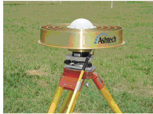
Antenna mounted on a wooden tripod.
