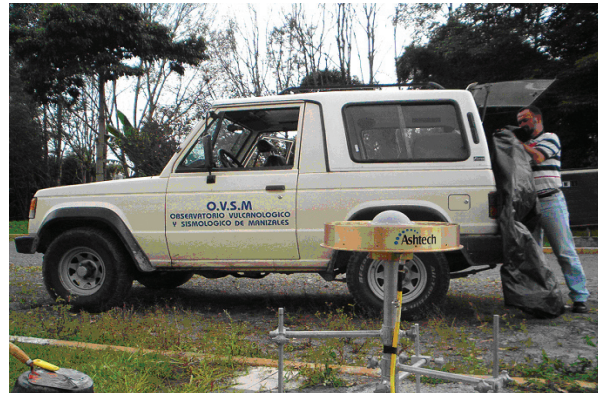
Installation of a GPS antenna on a constant-height base.
