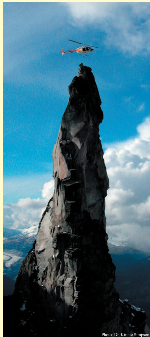
Figure 2: Helicopter with attached differential GPS antenna hovers over a distinctive rock formation, used as a ground control point for creation of a DEM. Data collection at this point took about 10 seconds.
