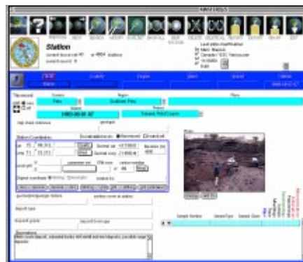
MAP db: Station window data layout: users can input field photographs and geological observations and can perform a number of location coordinate conversions.
